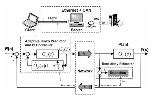
Figure 9 – Practical delay measurement approach (Lai and Hsu 2010) of remote control system.
