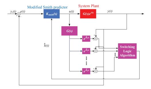
Figure 1.1 – Delay estimation and control diagram of the multi-model based technique (Herrera and Ibeas 2012).
