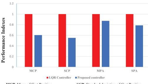
MCP: Mean of Cart Position MPA: Mean of Pendulum Angle **SCP**: Standard deviation of Cart Position **SPA**: Standard deviation of Pendulum Angle
