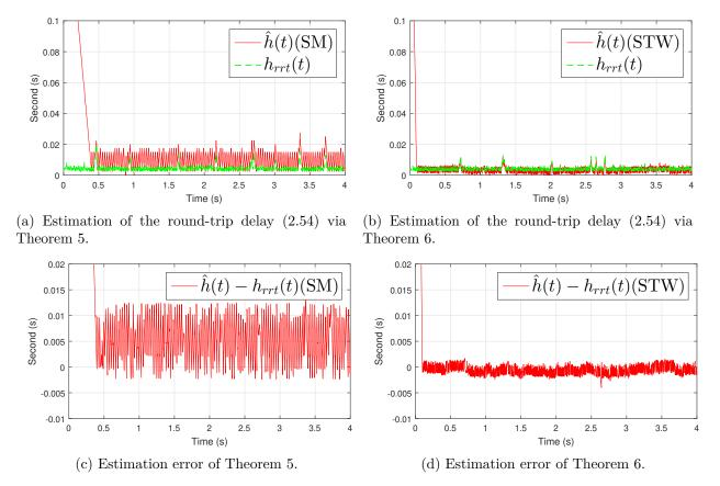
Figure 2.5 – Delay estimations and estimation errors of the round-trip delay (2.3) by using Theorems 5-6.
