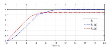
(a) Unknown time-delay h=6s, delay estimator  $\hat{h}_1(t)$  (with  $u_1(t)=\sin(t)$ ), and delay estimator  $\hat{h}_2(t)$  (with  $u_2(t)=e^{-2t}$ ) versus time.
