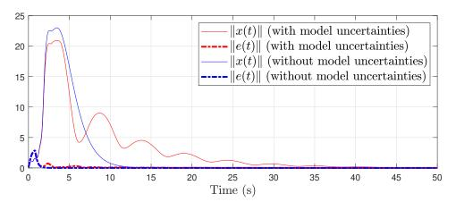
(a) System state x(t) and observation error e(t) of the nominal system (1.158) and the uncertain system (1.160) under control solution of Theorem 4 with initial condition  $\hat{h}(0) = 0.4$ s.
