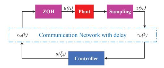
Figure 3.1 – General control diagram of networked control systems.
