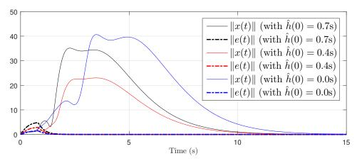
(a) System state x(t) and observation error e(t) of the system (1.158) under control solution of Theorem 4 with initial conditions  $\hat{h}(0) = 0.0$ s,  $\hat{h}(0) = 0.4$ s, and  $\hat{h}(0) = 0.7$ s.
