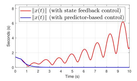
Figure 4 – State evolution of system (17) with state feedback control and predictor-based control.
