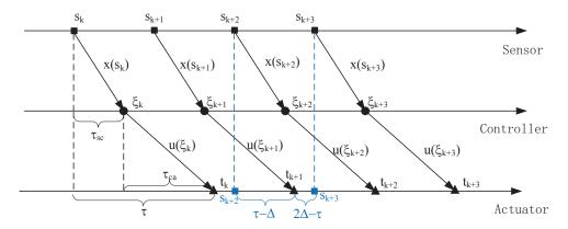
Figure 3.2 – Timing diagram of networked control system with constant delays.
