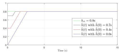
(b) Delay estimation of the system (1.158) under control solution of Theorem 4 with initial conditions  $\hat{h}(0) = 0.0$ s,  $\hat{h}(0) = 0.4$ s, and  $\hat{h}(0) = 0.7$ s.
