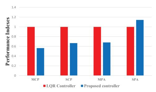
MCP: Mean of Cart Position MPA: Mean of Pendulum Angle **SCP**: Standard deviation of Cart Position **SPA**: Standard deviation of Pendulum Angle
