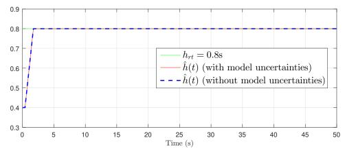
(b) Delay estimation of the nominal system (1.158) and the uncertain system (1.160) under control solution of Theorem 4 with initial condition  $\hat{h}(0) = 0.4$ s.
