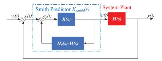
Figure 2 – Control diagram of the Smith predictor (Smith 1959).
