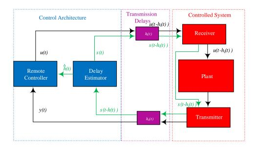
Figure 2.1 – Framework of the practical delay estimation techniques.
