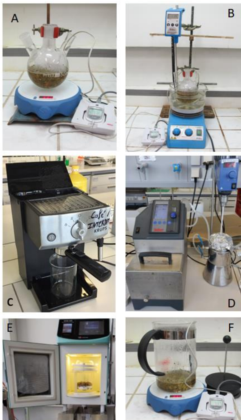
Figure SI-II.2. Picture of the experimental set-up used for each extraction mode (A: infusion; B: maceration; C: percolation; D: ultrasonic; E: Microwave; F: infusion using a French-Press Bodum® (with or without stirring)).
