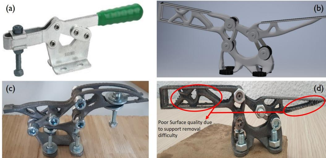
Figure 5.17: Tests with engineering students: (a) Generic clamp; (b) Topology optimized clamp; (c) Manufactured considering optimal orientation; (d) Manufactured without considering optimal orientation.
