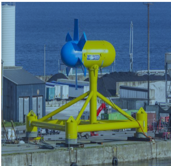
(a) Turbine Sabella [73]
