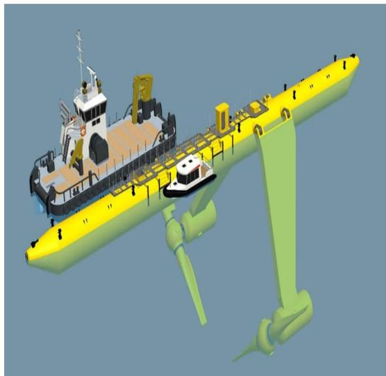
(b) Hydrolienne marine flottante - FloTEC, Scotrenewables Tidal Power [3, 4]
