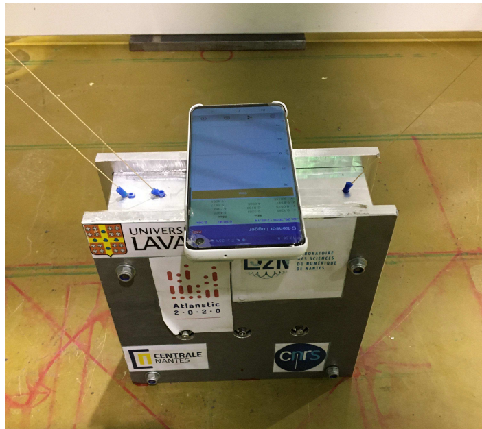
Figure 2.29: Measurement of the inclination \theta_n of the CDPC moving-platform with the accelerometer of a mobile phone
