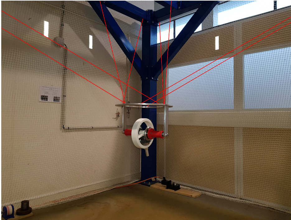
Figure 3.1: Prototype of the CDPR with an embedded tilt-roll wrist
