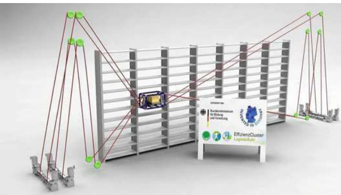
Figure 1.10: CABLAR CDR as a large-scale storage retrieval machine [ Bru+13b ; Bru+13a ; LBS13 ]
