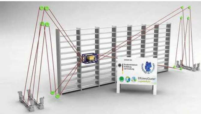
Figure 1.10: CABLAR CDPR as a large-scale storage retrieval machine [ Bru+13b ; Bru+13a ; LBS13 ]
