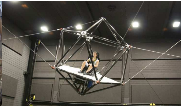
Figure 1.15: The CableRobot motion simulator with a large translation workspace, [Mie+16]
