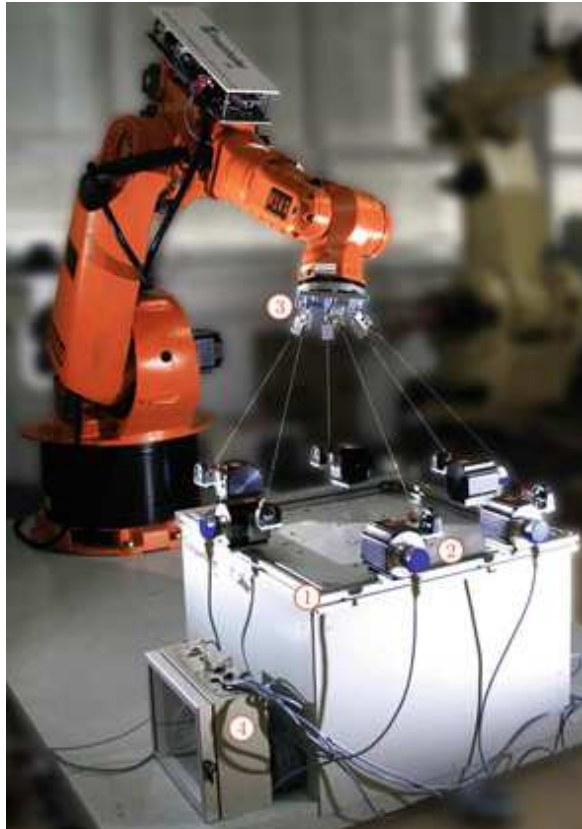
Figure 1.12: IPAnema 2 measurement device: Cable sensor based 6-DoF pose measurement system applied to measure the pose of an industrial robot, [Pot+13]
