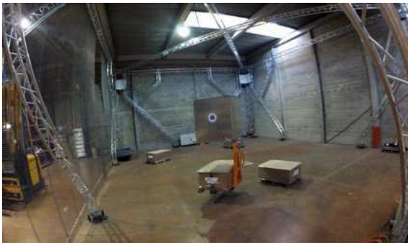
Figure 1.14: Prototype of the CDPR with large translation workspace in the context of the CoGiRo project, [Gou+15b]
