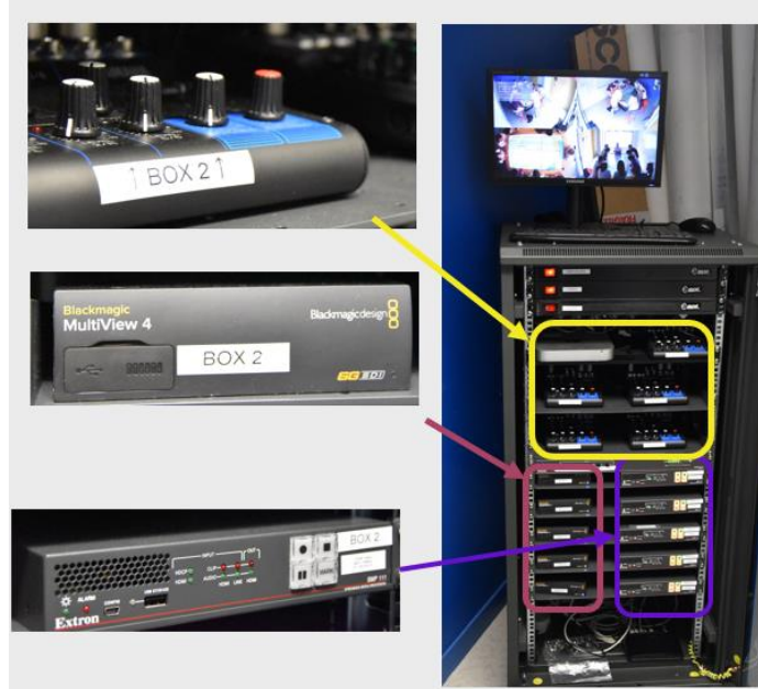
Figure 35: Video and audio capture system
