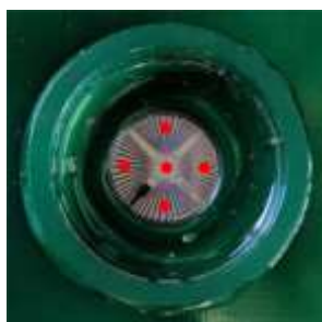
Figure 67 : Photo of MEA-1 with red dots representing the positions where fluorescence and temperature were recorded (i.e. electrodes area, upper lines, lower lines, right lines, left lines).
