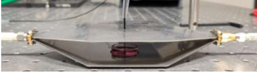
Figure 9 : Open TEM cell used for in vitro Bioelectromagnetic studies.
