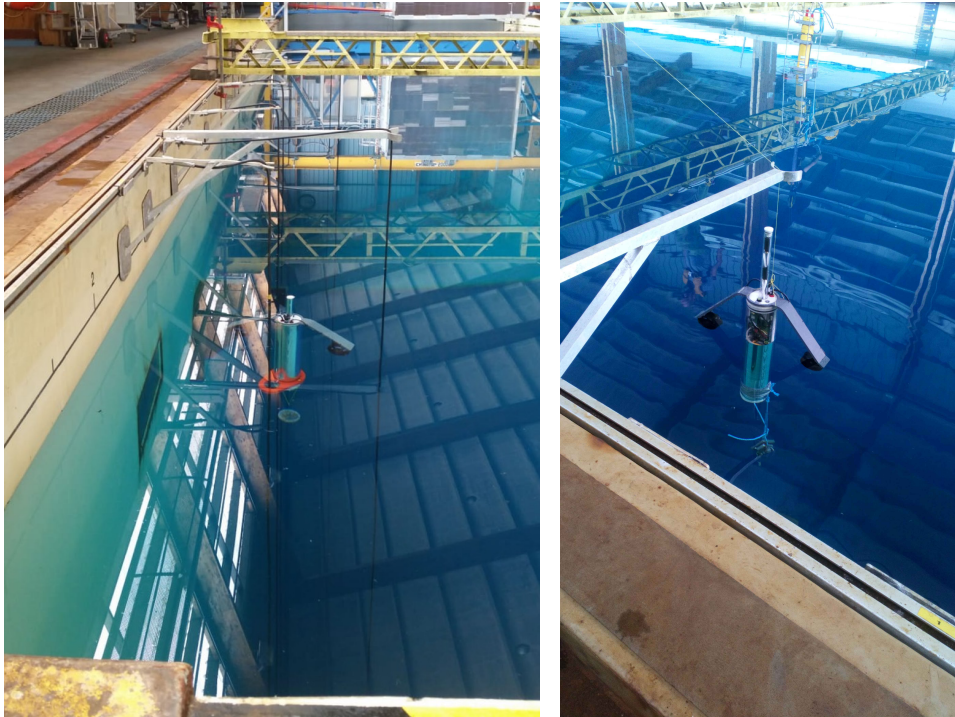
Figure 5.12: Ifremer Brest water tank with the SeaBot float. The robot is secured along a rope guide.
