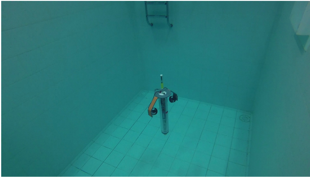
Figure 5.16: Last test of the SeaBot depth controller in the ENSTA Bretagne 2.5m deep pool before a deployment in the Bertheaume cove. Note that we added colored stripes to make it easier to find the robot at the end of the mission.
