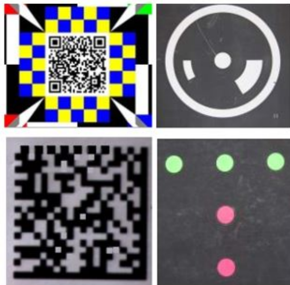
Figure 1.14: Four examples of coded targets used for point identification and camera calibration [Maut 11]
