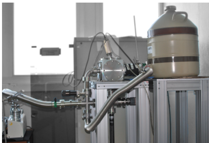
Figure 2.1 – Experimental set-up for \beta spectrometry, developed at LNHB in 2012.
