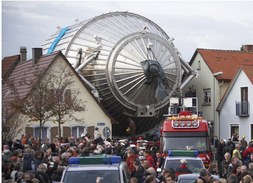
Figure 1.15 – The KATRIN spectrometer, built to measure the mass of the antineutrino particle with sub-eV precision by measuring the \beta spectrum of tritium, being moved to the Karlsruhe Institute of Technology (KIT).
