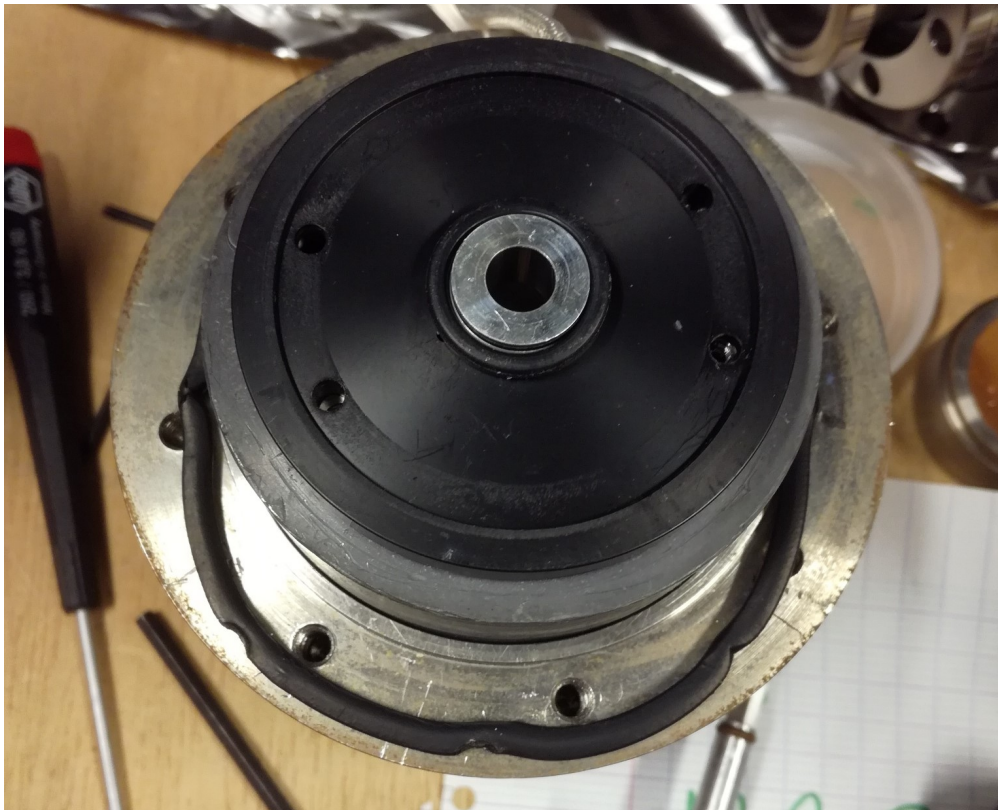
FIGURE 4.15: Photograph of a disassembled part of the spectrometer, showing a damaged o-ring.
