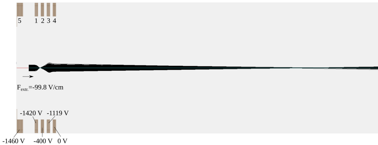
FIGURE 4.17: Electron trajectories simulated in the Simion software under low extracting field ( F_{extr.} = -99.8 \text{ V/cm} , created by V_5 = -1460 \text{ V} and V_1 = -1420 \text{ V} ) and optimal tuning of potentials 2 and 3 ( V_2 = -400 \text{ V} and V_3 = -1119 \text{ V} ). Note the crossover ten centimetres away from the output of the electron source, corresponding to a virtual source a few centimetres in front of the apertures of the spectrometer. This configuration corresponds to the circled data point in figure 4.18.
