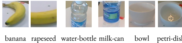
Figure 2.20: Object labels for different sample patches using a pre-trained CNN ( AlexNet ). It often fails when patches contain only partial views of objects (banana and water bottle) or unexpected points of view (bowl).
