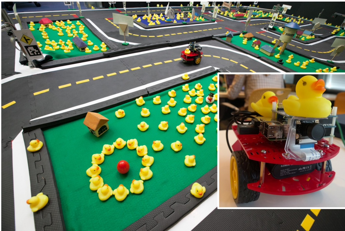
Figure 2.4: Duckietown is a scaled-down autonomous city where the inhabitants are duckies. The platform comprises autonomous vehicles (Duckiebots) and a well-specified environment in which the Duckiebots operate. This platform is used as the basis for the AI Driving Olympics competition which will take place at the NIPS 2018 conference.
