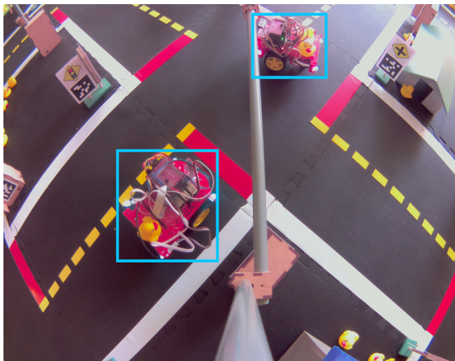
Figure 2.9: The overhead cameras are used to provide ground truth localization of the robots inside the Robotarium environments.
