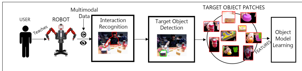
Figure 2.12: Object model learning from human-robot interaction. In the proposed pipeline the user interacts with the robot for it to learn new object models. We capture audio and video from this interaction. The data is processed to recognize the interaction type which guides the segmentation of the target object patches in the images. These patches are used to learn new object models.
