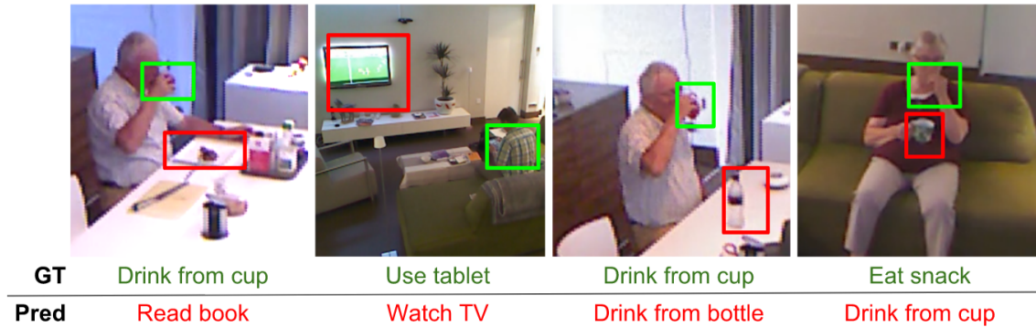
Figure 6.1: Separable STA correctly discriminates the activities with fine-grained details. The model without attention (I3D) is misled by imposter objects (displayed in red boxes) in the image whereas our proposed separable STA manages to focus on the objects of interest (displayed in green boxes).
