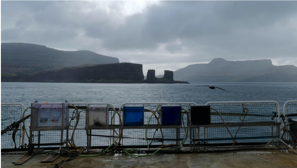
Fig. B3: Picture of the on-deck incubators in the vicinity of the Kerguelen islands. In situ temperature was reproduced in the incubator by a constant flow of sub-surface seawater. In situ light intensity of the sampling depth (10 m) was mimicked using blue light screens attenuating direct sunlight by approximately 50%.
