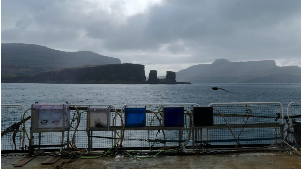
Fig. B3: Picture of the on-deck incubators in the vicinity of the Kerguelen islands. In situ temperature was reproduced in the incubator by a constant flow of sub-surface seawater. In situ light intensity of the sampling depth (10 m) was mimicked using blue light screens attenuating direct sunlight by approximately 50%.
