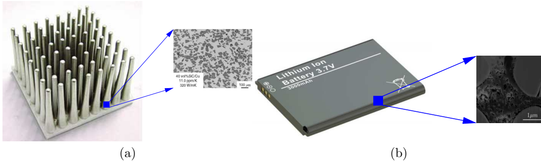
Figure 1.1: Engineering applications of transient diffusion phenomena using heterogeneous materials. (a) The heat sink material for the processor of a computer, the irregularly shaped silicon-carbide particles are embedded in a copper matrix [1, 2]. (b) The electrolyte-electrode system of a lithium-cobalt-oxide battery, the large circular active particles are embedded in the matrix [3, 4].
