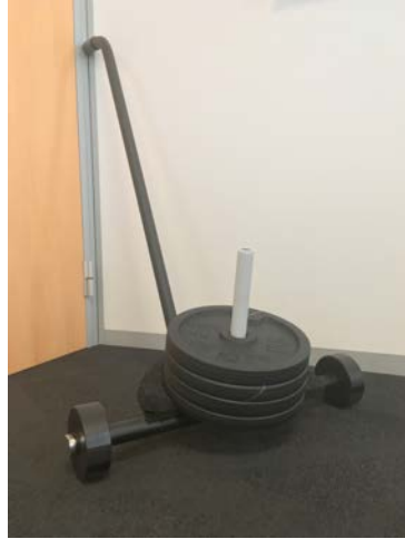
Figure 4.9: Test trolley used for model validation tests: shown here with 20 kg added mass.
