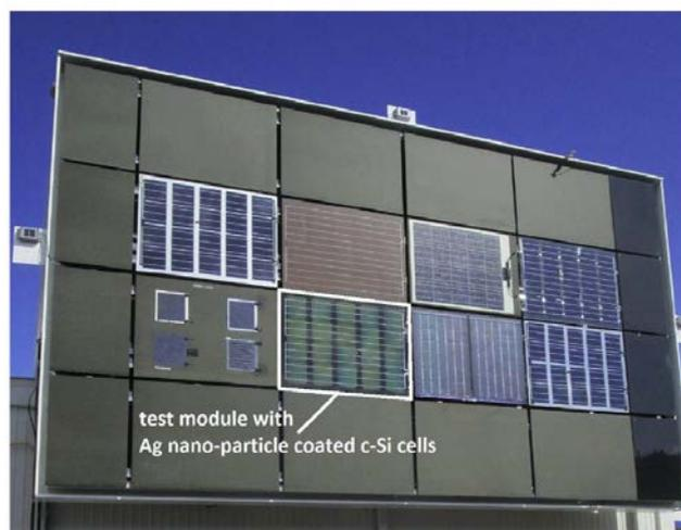
FIGURE 1.17 – Exemples de modules PV colorés (« Application of Plasmonic Coloring for Making Building Integrated PV Modules Comprising of Green Solar Cells » 2017)
