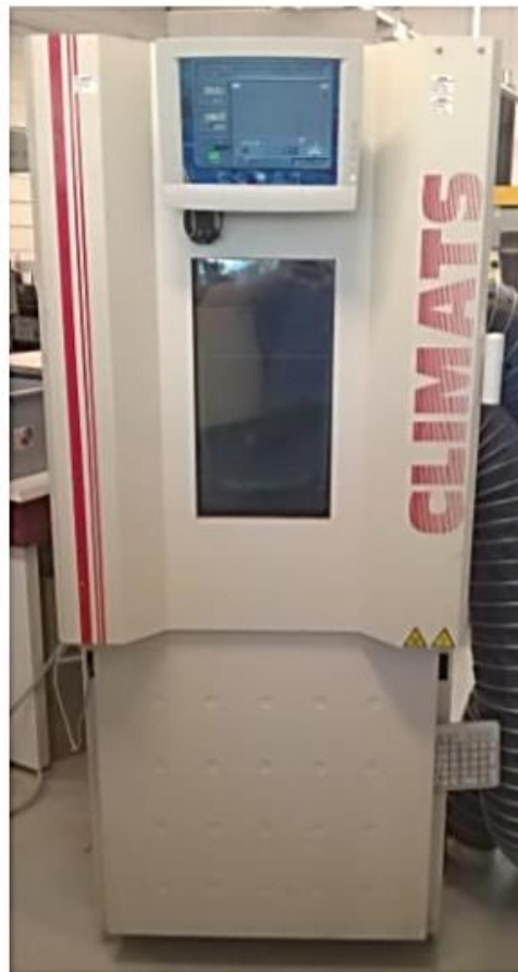
Figure 5.23: Climatic chamber CLIMATS Type EX2221-HA.
