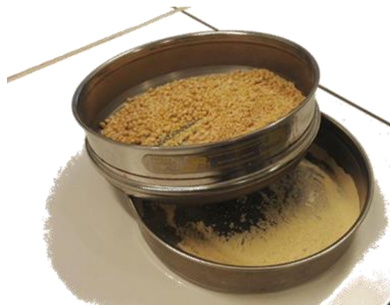
Figure 4.18: Sieving of the finer fraction (smaller than 0.400 mm) of the crushed soybeans powder.
