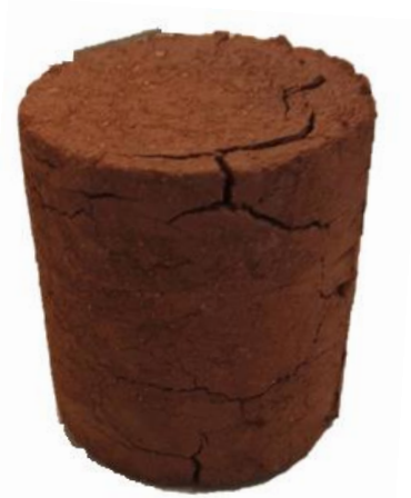
Figure 6.22: Formation of cracks after spraying the whole amount of cementing solution (equal to 80 % w_L ) on the sample surface in a single application.
