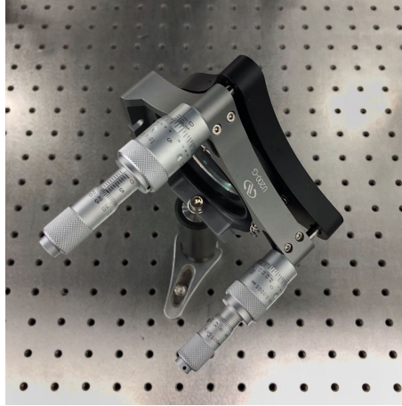
Figure 6.14 Alignment mirror mounts implemented with actuators which could realize sub-micron resolution of tuning used in preliminary TBOX experimental setup.
