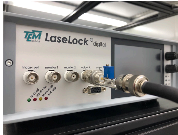
Figure 6.13 A potentiometer (BOURNS 3296, in color blue) with resistance range from 10 ohm to 2 megaohm is implemented in the cable connecting the output of LaseLock with the input of Koheras piezo port to successfully remove the noises as shown in Fig. 6.12 and resulted in clean signals as shown in Fig. 6.11.
