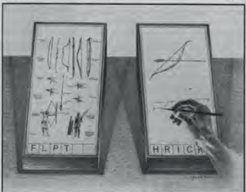
MEMEX IN USE is shown here. On one transparent screen the operator of the future writes notes and commentary dealing with reference material which is projected on the screen at left. Insertion of the proper code symbols at the bottom of right-hand screen will tie the new item to the earlier one after notes are photographed on supermicrofilm.
