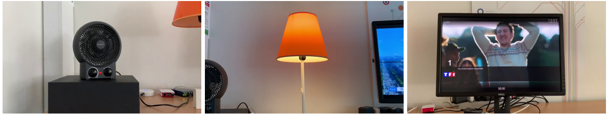
Figure 8.5: Illustration of the objects used to showcase the system. The fan (Left) was connected to a smart plug and the connected Light (Middle) and could be turned ON or OFF with a single command. The television (Right) could be controlled using a hierarchical menu.
