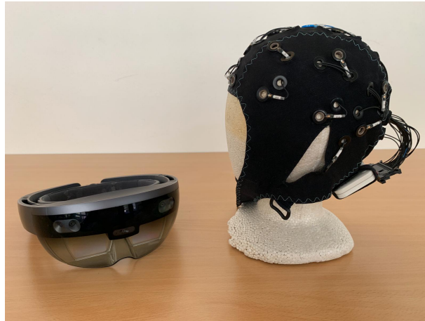
Figure 8.4: Illustration of the apparatus used in the developed prototype. (Left) A Microsoft HoloLens and (Right) an mbt Smarting.
