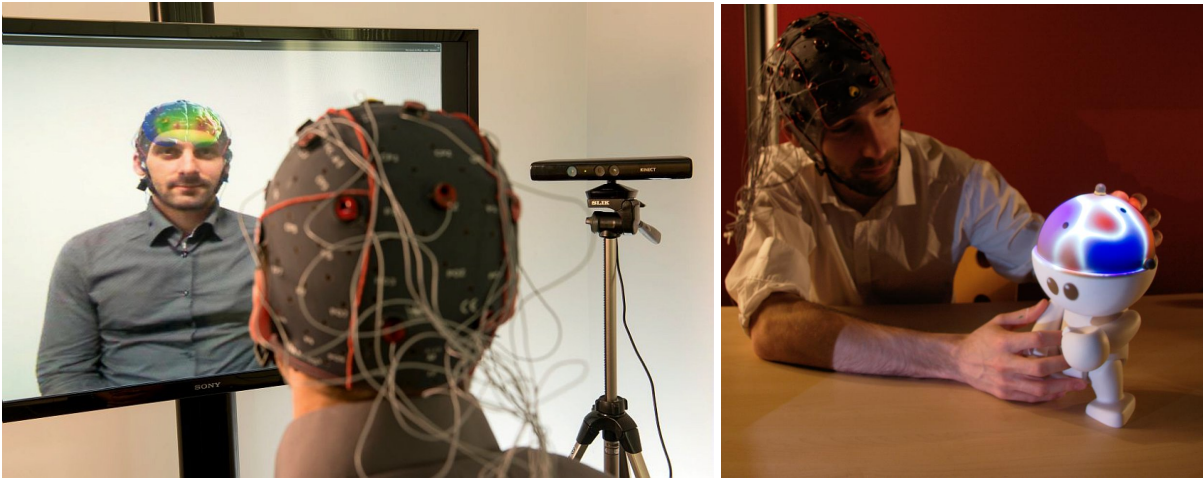
Figure 2.5: Examples of works combining BCI and AR for brain activity visualization. (Left) represents the Mind Mirror a system displaying the user's brain activity in a smart mirror for neurofeedback [Mercier-Ganady et al., 2014]. (Right) displays an example of SAR combined with BCI for brain activity visualization. The brain activity of the user is displayed on the brain of Teeg a pedagogical robot for teaching EEG [Frey et al., 2014].
