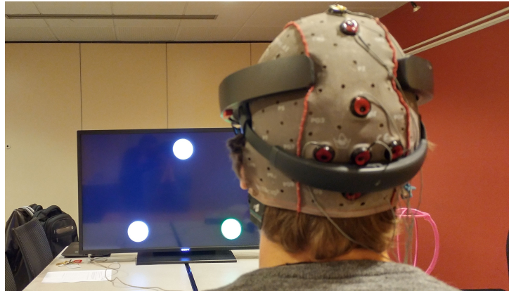
Figure 4.1: Experimental setup of Study 1: the user wears an EEG cap as well as the HoloLens. In this particular condition, the SSVEP targets were displayed on the screen.
