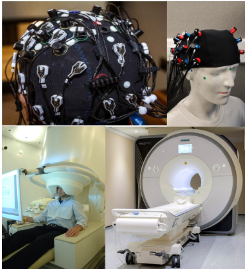
Figure 1.6: Examples of brain activity measurement devices namely: an EEG (top left), an fNIRS (top right), an MEG (bottom left) and an fMRI (bottom right) 6 .
