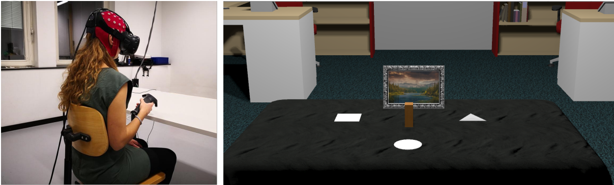
Figure 5.1: Experimental setup used in our study. Left : participant wearing both an EEG cap (ANTNeuro EEGO sports) and an HTC Vive VR headset. Right : virtual environment. Participants were seated in front of a virtual table on which three targets were displayed. The virtual object (brown) was placed in the middle of the three targets and had to be picked up and placed on one target.
