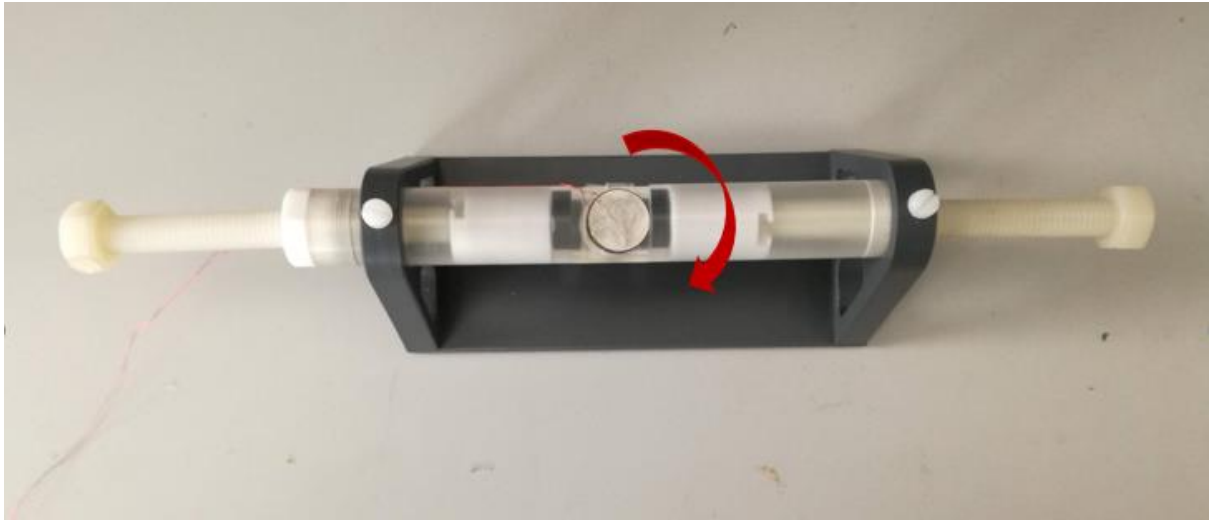
Figure 2.18- Top view of the sample's holder with the ME composite.
