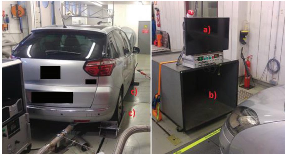
Figure 2.3. Chassis dynamometer device: a) screen; b) fan; c) roller bench system.
