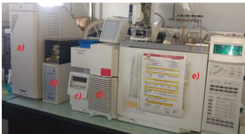
Figure 2.13. TD-GC-MS analytic system, a) sample changer, b) thermo-desorber, c) air server, d) mass spectrometer, e) gas phase chromatograph.
