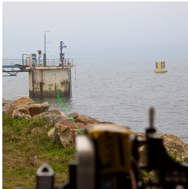
Figure I.5: Testing of surface elevation measurement using a lidar camera with grazing incidence at Ifremer, Brest, in November 2018. This image corresponds to the calibration phase of the instruments; during the measurements the laser target point was located on the right side of the tower, below a ultrasound wave probe that was used to provide data to compare with. Credit: ECN.
