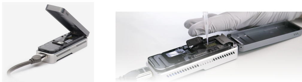
Figure 2.10: The MinION nanopore sequencer by Oxboard Nanopore Technologies 2
