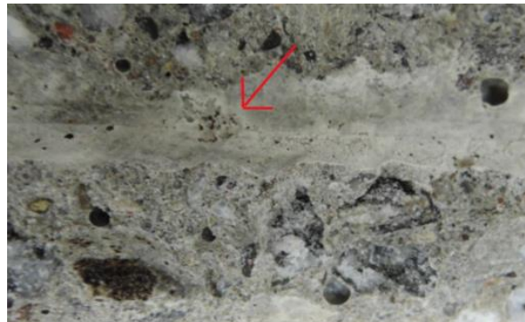
Figure II-51 Examples of irregularities at the steel-concrete interface Locally higher porosity (arrow) and small air voids (left part) as well as coarse air voids (right part). Corrosion initiated in this case at the arrow[139]
