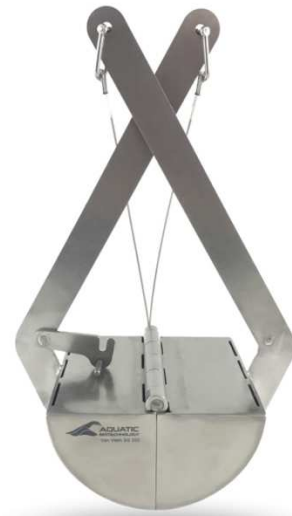
Fig. II.2 Van Veen grab dredging device
