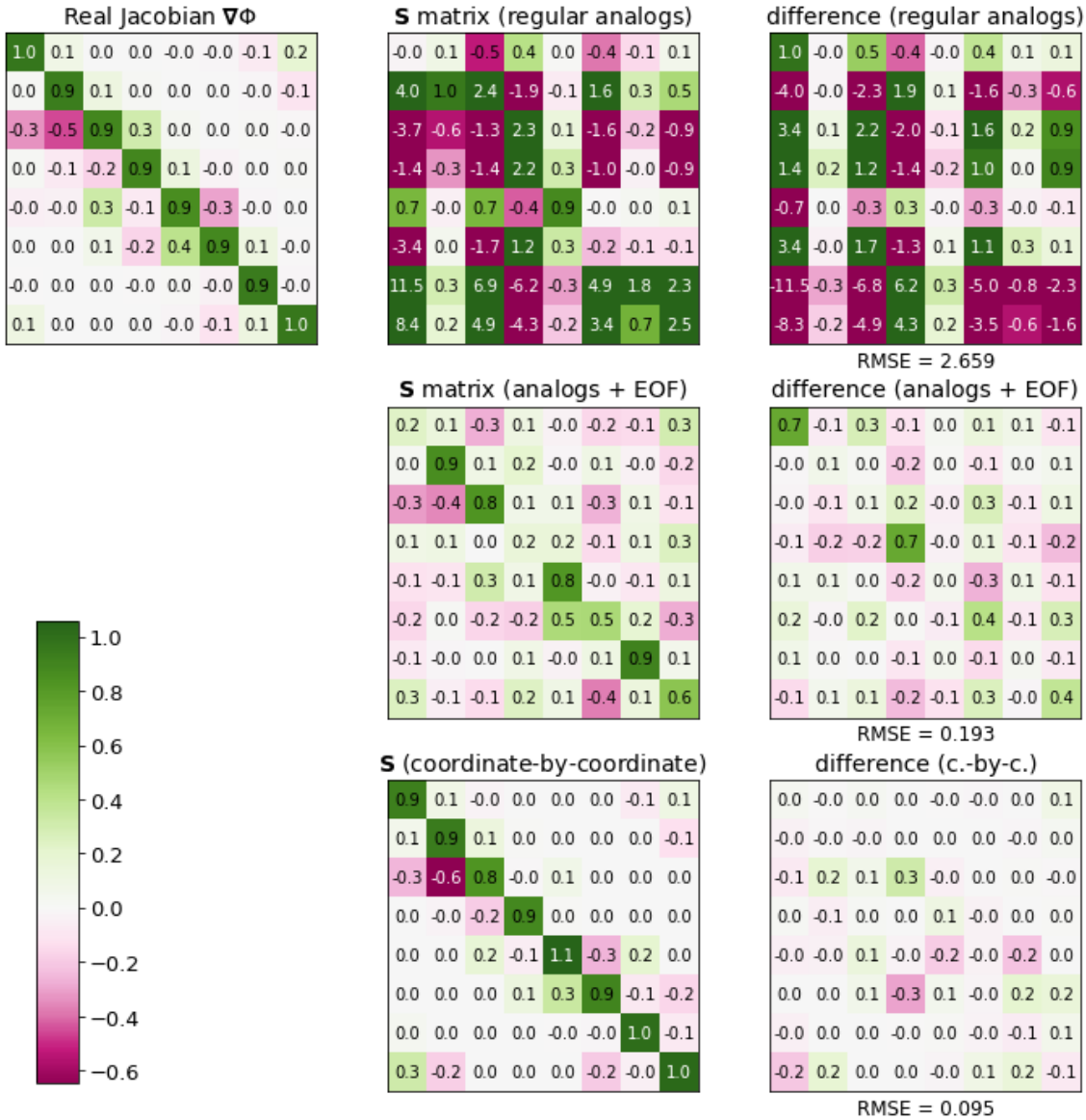
Figure III.3: Flow map Jacobian matrix estimation with the model of Lorenz (1996). Forecast lead time is t = 0.05 Lorenz time, catalog length is 10^4 Lorenz times, phase-space dimension is n = 8 . K = 9 analogs are used for the forecast and Gaussian kernels for the weights \omega_k with shape parameter \lambda set to the median of analog-to-state distances |\mathbf{a}_0^k - \mathbf{x}_0| . Upper-left: Jacobian matrix \nabla\Phi^t|_{\mathbf{x}_0} . Upper-middle: linear regression matrix \mathbf{S} using regular analogs. Upper-right: difference \mathbf{S} - \nabla\Phi^t|_{\mathbf{x}_0} with regular analogs, also giving the value of RMSE below the plot. Middle panels: same but the linear regression is performed in a lower-dimensional subspace spanned by the first EOFs of the set of the K = 9 analogs. Lower panels: same but the linear regression is performed coordinate-by-coordinate, and assuming that the coefficients are zero two cells away from the diagonal.
