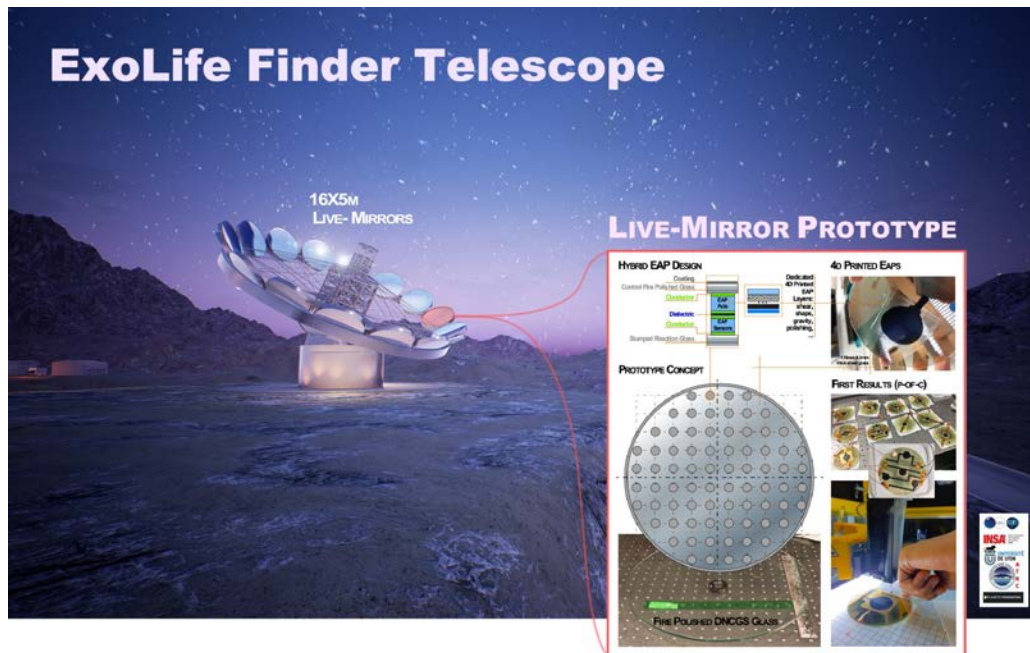
Figure 85 Efforts to make “Live-Mirror” prototype a reality have been our Live-Mirror project team goal. R&Ds for a precise and smooth optical surface controlled by an active and live system via 3D-Printing of force actuators should pave the way for future development of the next-generation telescope mirror dedicated and optimized for high-contrast observations – Exo-Life Finder Telescope.
