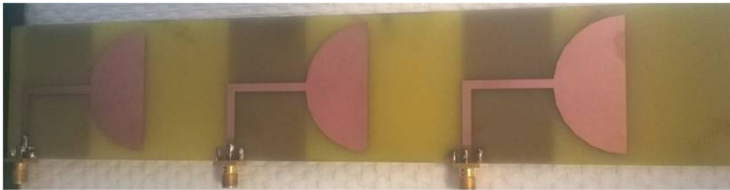
Figure 4-31: First prototype of the SPYBOAT® antenna array
