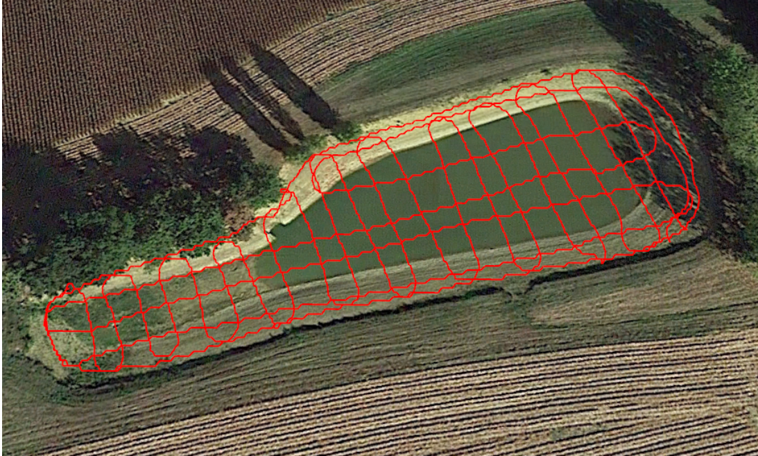
Figure 5-8: Example of plane trajectory achieved by a SPYBOAT® SWAN vehicle in manual mode during a bathymetric survey
