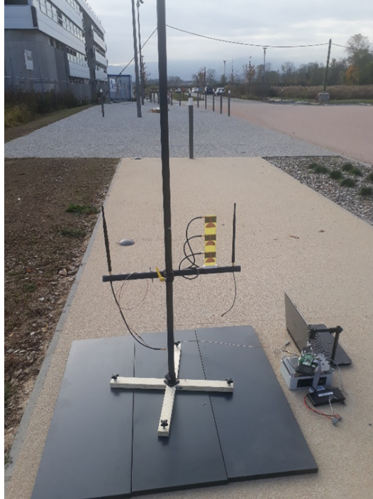
Figure 4-33: Fiberglass support fabricated for measurements
