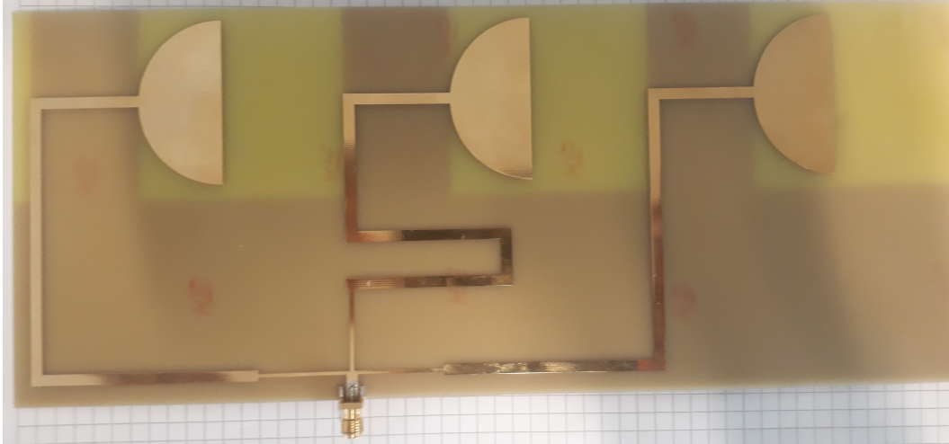
Figure 4-38: Complete antenna prototype
