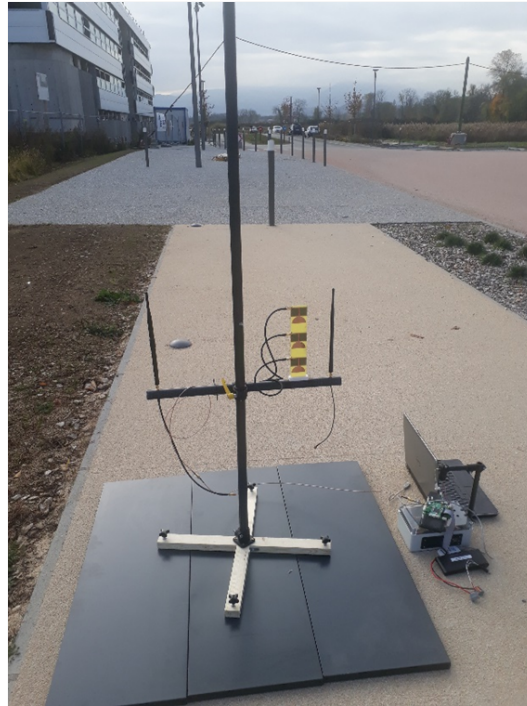
Figure 4-33: Fiberglass support fabricated for measurements
