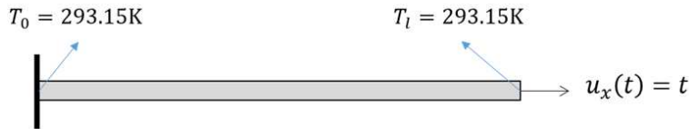
Figure 3.17. – 2D clamped beam for the thermoelastic problem
