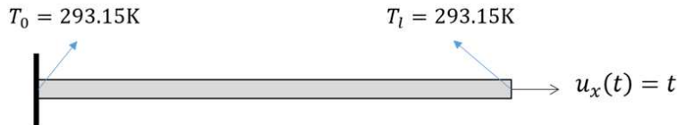
Figure 3.17. – 2D clamped beam for the thermoelastic problem
