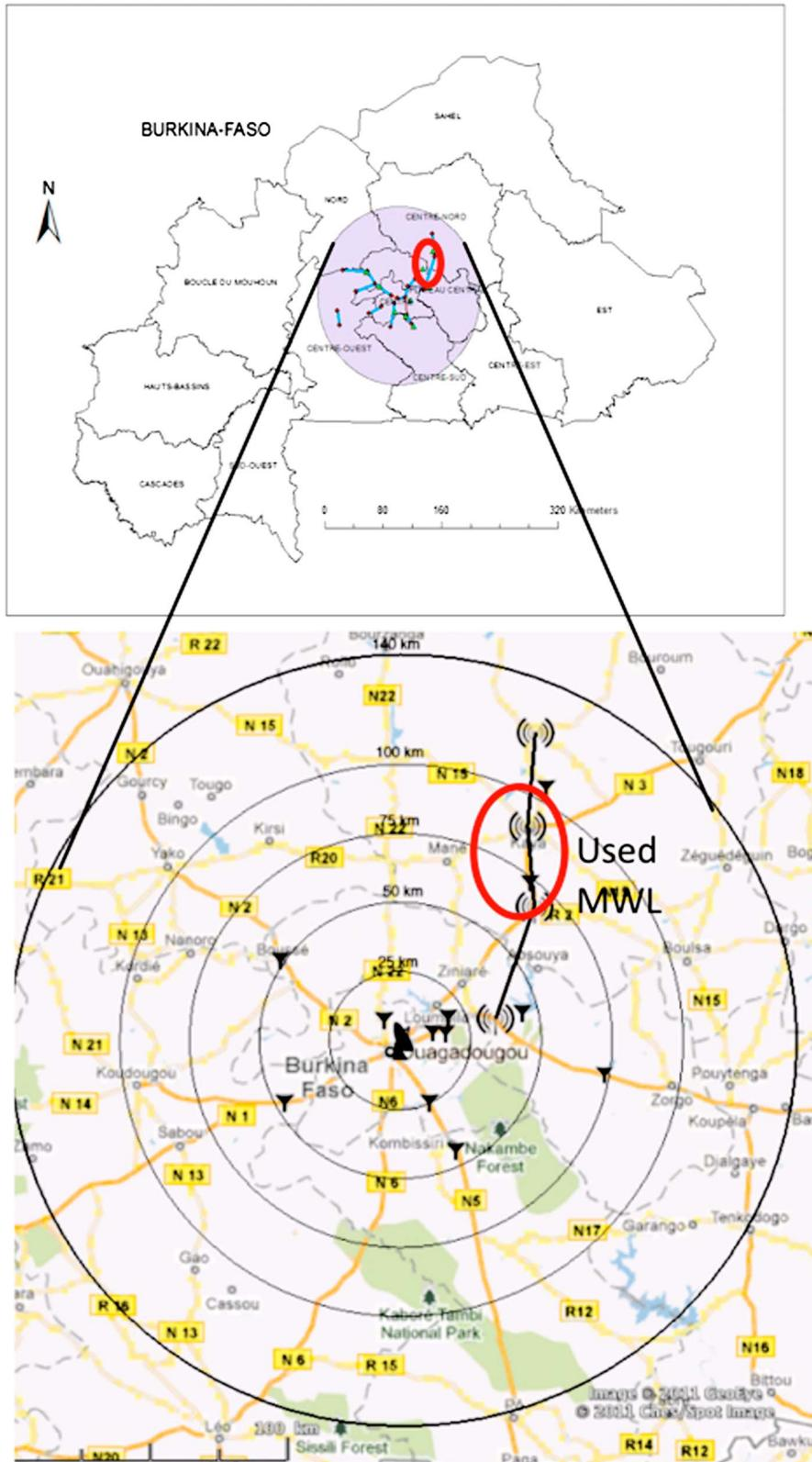
**Figure 1.** Location of the study area in Burkina Faso and instrumental setup. The red ellipse shows the Korsimoro-Kaya link and the Boussouma rain gauge used for this study. The purple circle and the blue segments are for the X band radar and link network that will be available for the analysis of the 2013 season.
