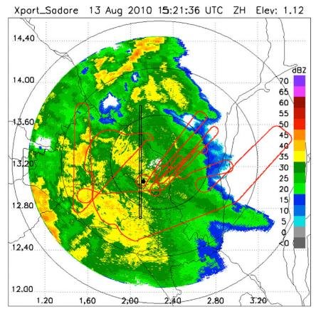
FIG. 1. Xport radar reflectivity field (1.12° elevation) for 1521:36 UTC 13 Aug 2010. Red line: ground projection of the instrumented-aircraft trajectory for the flight (which lasted from 1323 to 1610). The black rectangle is the ground projection of the volume used to analyze the time evolution of the microphysics (section 5), and the black point is the position of the Deberegati rain gauge (13.058°N, 2.122°E).
