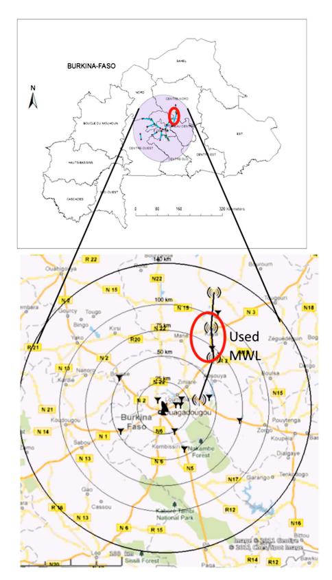
**Figure 1.** Location of the study area in Burkina Faso and instrumental setup. The red ellipse shows the Korsimoro-Kaya link and the Boussouma rain gauge used for this study. The purple circle and the blue segments are for the *X* band radar and link network that will be available for the analysis of the 2013 season.
