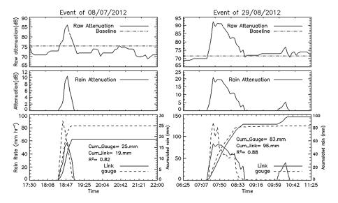
**Figure 4.** Five-minute resolution time series for two events (date as title). (a) Solid line: raw microwave attenuation (reception minus transmission). Dotted line: baseline (dry) attenuation. (b) Path attenuation due to rain. (c) Solid line: rain rates estimated from link. Dashed line: gauge rain rates.
