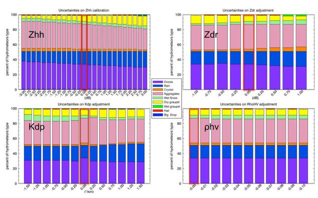
FIG. 3. Sensitivity of HID algorithm to the uncertainty in each radar variable (see text). The y axis is percentage of each hydrometeor, and the x axis is the bias applied to each radar variable, as indicated. The test is applied to the volume scan acquired 1606 UTC 13 Aug 2010. The highlighted red rectangles show the default setup of the HID algorithm.
