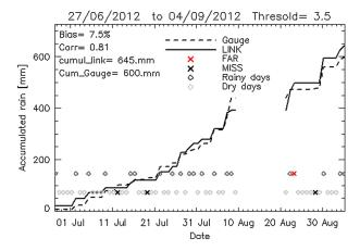
**Figure 3.** Cumulated daily rainfall series from the gauge (dash line) and the link (plain line). The black diamonds mark the days with correct detection of rain, the red cross for the false alarm (of the link compared to the gauge), the black cross for the missed rain, and the gray diamonds for the days with no rain detected by any sensors.
