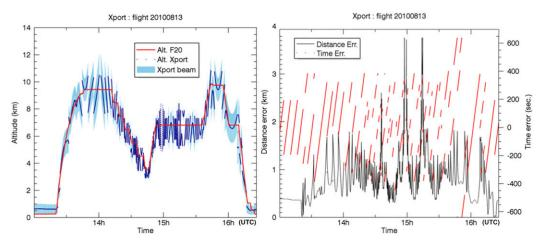
FIG. 5. (left) Altitude vs time for the aircraft (in red) and the closest radar pixel (in blue) with associated radar beamwidth (in light blue). (right) Distance (in black) and time-sampling (in red) errors between the aircraft observations and the closest radar pixel (see text).
