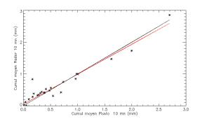
$\texttt{Étalonnage}: 1.3 \text{dB, Ratio} = 0.948, \, R^2 = 0.939, \, \text{Nash} = 0.937, \, \text{RMSE} = 0.151 \quad \text{Nbias} = 0.055$
