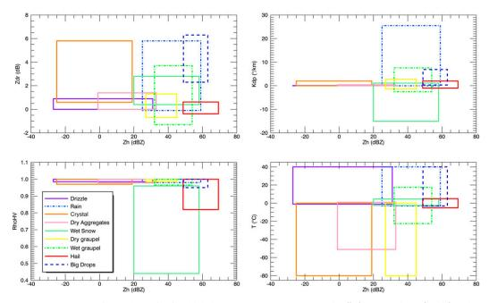
FIG. 2. Representation of the region in which the MBF of  $Z_{DR}$ ,  $K_{DP}$ ,  $\rho_{hv}$ , and T (°C) are equal to 1 (y axis) vs the one in which the MBF of  $Z_h$  is equal to 1 (x axis). The colors and line styles are for the nine hydrometeor types, as indicated.
