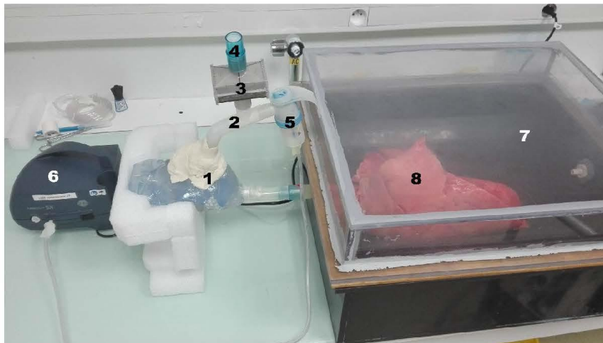
40 Figure 2 – Photographic image of the ex vivo model before the nebulization of SRP. 1: ENT. 2: Mouthpiece. 41 3: Expiratory filter. 4: One-way valve for exhalation. 5: Nebuliser. 6: Compressor. 7: Sealed enclosure. 8: 42 Porcine respiratory tract.
