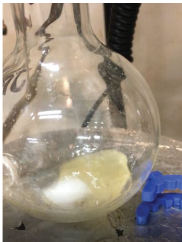
Figure II. 60: Increase of viscosity observed at the mix of poly(styrene-co-4-vinylpyridine) and B(C_6F_5)_2 -Ph- B(C_6F_5)_2 with 2 molar equivalents of triethylamine in toluene.
