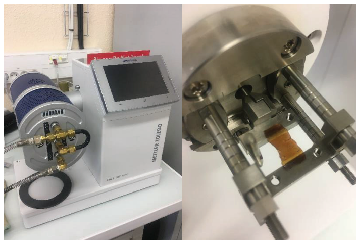
Figure IV. 72: Left: DMA device; Right: Experimental set up of the sample.
