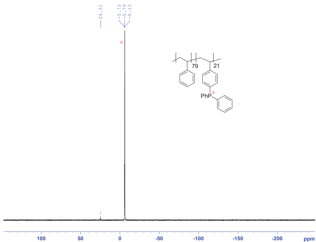
Figure V. 32: ^{31}\text{P} NMR spectrum of poly(4-styryldiphenylphosphine-co-styrene) with 21 % mol of 4-styryldiphenylphosphine in the copolymer in \text{C}_6\text{D}_6 . * \text{C}_6\text{D}_6
