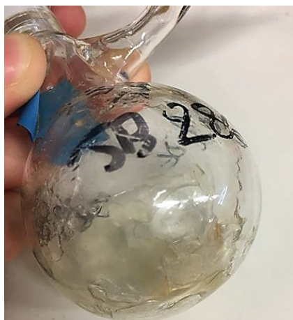
Figure II. 58: Recovery of gel after drying of the solution of poly(4-vinylpyridine) and B(C_6F_5)_2-Ph-B(C_6F_5)_2 in chloroform.
