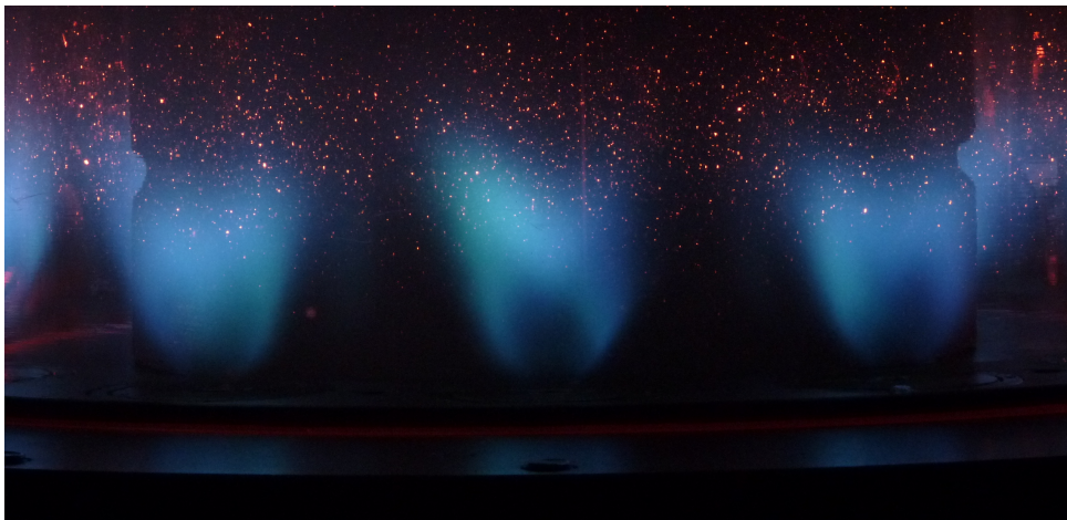
Figure 9.3: Direct chemiluminescence image of several stable flames in MICCA-Spray at operating point ( \mathcal{P} = 107 \text{ kW} , \phi = 1.04 , u_b = 33.4 \text{ ms}^{-1} ). The exposure time is 100 ms so that the images are time-averaged. The flames have a typical “M”-shape. Slight differences can be observed from one flame to the other. The system is not perfectly rotationally symmetric due to the presence of the spark plugs, and differences in fuel atomization between each injector.
