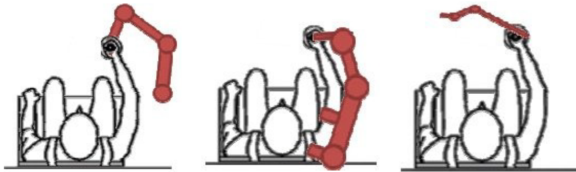
(a) co-manipulation Parallèle (b) co-manipulation Orthétique (c) co-manipulation Sérielle
