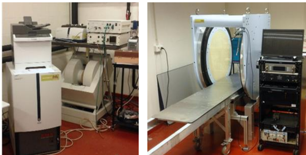
Figure 2-10. Examples of EPR instrumentation used in oximetry. Left: EPR X-band used for in vitro samples and, right: EPR clinical L-band used for in vivo work.
