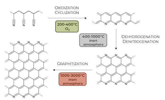
Figure 2.2 – Simplified process of PAN conversion to graphite-like layers Adapted from Huang, 2009
