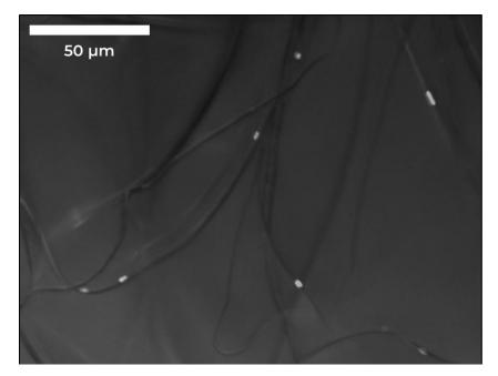
Figure 4.11 – Epifluorescence micrograph of coelectrospun fibers (shell: PCL 9 wt% + PEG 1 wt% in 90:10 (w/w) chloroform & DMF; core: PEO 5 wt% in PBS 0.5X + GFP-expressing *D. dadantii* at  $OD_{600} \approx 1$ ). The image is a composite of the brightfield and of GFP channels (the bacteria appear as the white dots).
