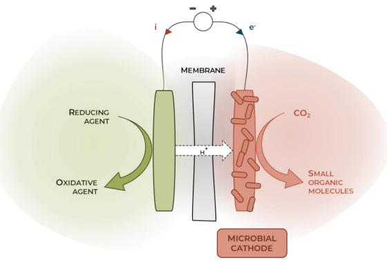
Figure 1.7 – General architecture of a microbial electrosynthesis cell
