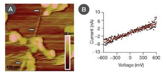
Figure 1.13 – Conducting-probe atomic force microscopy on *G. sulfurreducens* pili with (A) the topography of a pilus (indicated by arrows) and non-pilin globular proteins and (B) the correspondence between current and applied voltage on a section of the pilus.
