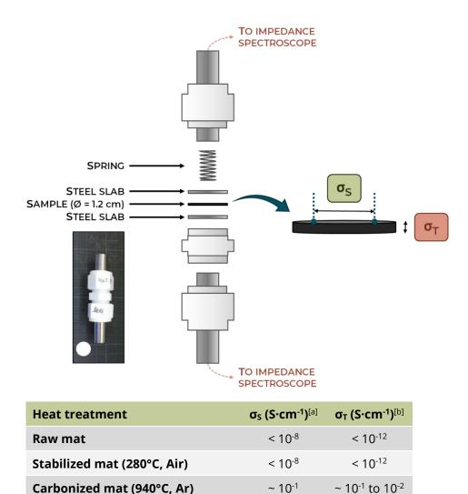
Figure 2.17 – Swagelok cell setup & typical electrical conductivities  $\sigma_s \& \sigma_T$  for the electrospun PAN membranes at different stages of the heat treatment (electrospun from a 10 wt% PAN in DMF solution, stabilized under air at 280°C, carbonized under argon at 940°C).
