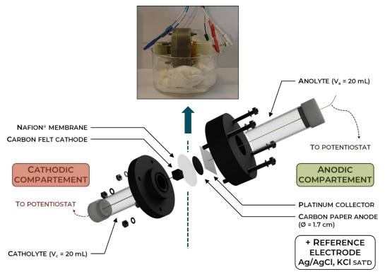
Figure 2.23 – Lab-scale two-compartment microbial fuel cell setup
