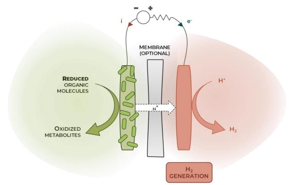
Figure 1.6 – General architecture of a microbial electrolysis cell
