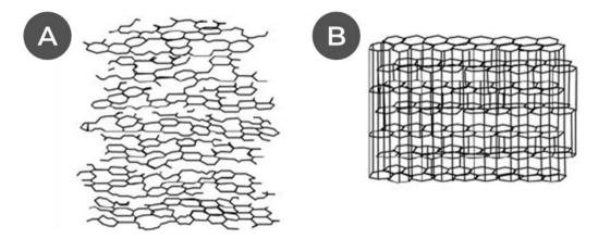
**Figure 2.4 – Schematic representation of (A) a turbostratic and (B) a graphitic carbon structure** Adapted from Dasgupta & Sathiyamoorthy, 2003
