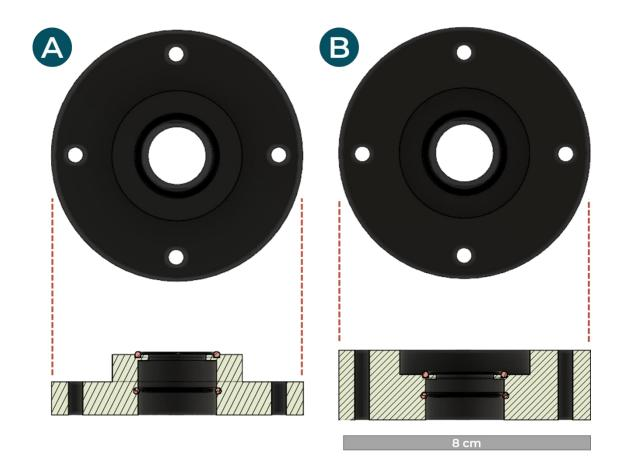
Figure A.6 – Radial cut of the 2 parts of the MFC reactor body: (A) Cathodic side; (B) Anodic side.
