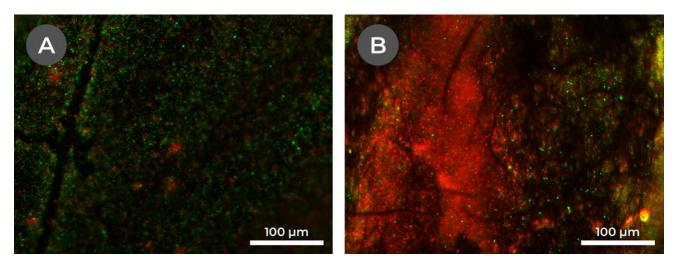
Figure 2.45 – Epifluorescence microscopy of the electrospun carbon electrode dyed with Invitrogen<sup>™</sup> LIVE/DEAD<sup>™</sup> BacLight<sup>™</sup> Bacterial Viability Kit (SYTO 9/Propidium iodide) (A) before & (B) after cryodesiccation. Green highlights live cells while red highlights dead cells.
