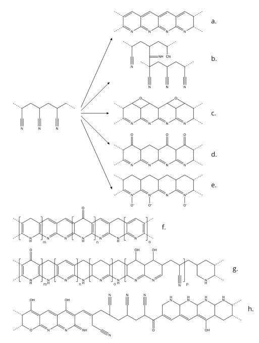
**Figure 2.3 – Proposed products of the oxidation/cyclization of PAN** Adapted from Huang, 2009
