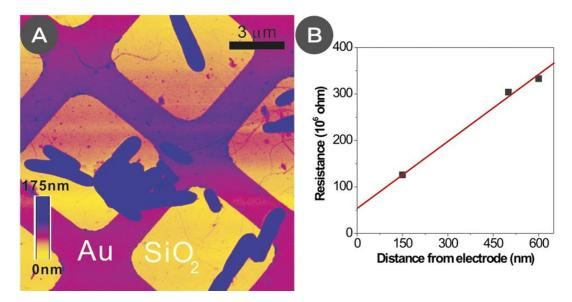
Figure 1.14 – CP-AFM of a bacterial nanowire with (A) the topographic AFM image showing airdried *Shewanella oneidensis* MR-1 cells and extracellular appendages deposited randomly on a SiO<sub>2</sub>/Si substrate patterned with Au microgrid and (B) a plot of total resistance as a function of distance between AFM tip and Au electrode.
