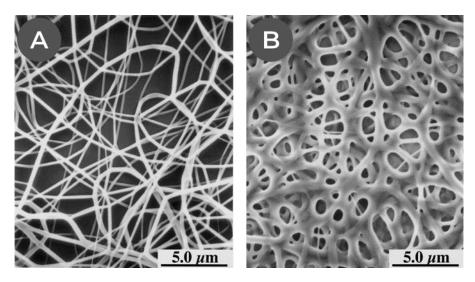
Figure 1.34 – SEM micrographs of electrospun nylon 6-6 in formic acid at (A) 2.0 cm & (B) 0.5 cm. Adapted from Uyar & Besenbacher, 2008
