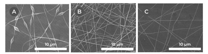
Figure 1.31 – Influence of the net charge density changes due to the addition of NaCl on the architecture of PEO in water electrospun fibers. The electric field is 0.7 kV/cm. The weight fraction of PEO is 3 %. (A) 1.23  $C \cdot L^{-1}$ ; (B) 6.57  $C \cdot L^{-1}$ ; (C) 28.8  $C \cdot L^{-1}$ .
