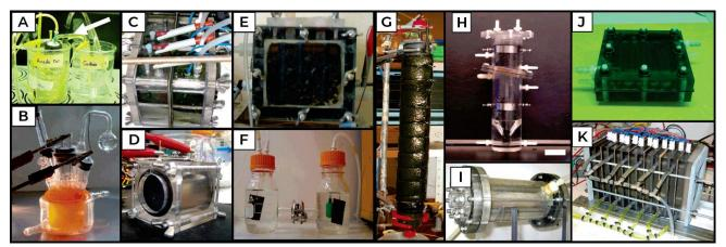
Figure 1.20 – Types of (A)–(F) lab-scale & (G)–(K) continuous operation MFCs. (A) Salt-bridge type; (B) Photoheterotrophic type; (C) Four batch-types separated by a membrane; (D) Single-chamber with air cathode; (E) Batch-type; (F) Two-chamber H-type with gas sparging; (G), (H) Upflow tubular type; (I) Single-chamber with inner concentric air cathode; (J) Flat-plate design with serpentine pattern design inside; (K) Stacked MFCs with 6 MFCs joined in a block.
