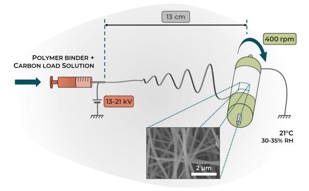
Figure 3.3 – Overview of a composite electrospinning setup.
