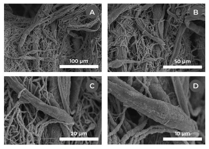
Figure 4.25 – SEM micrographs of an air-dried post-mortem integrated bioanode (shell: PCL 6 wt% + PEG 1.5 wt% + CB 2 wt% in 90:10 (w/w) chloroform & DMF; core: PEO 5 wt% in PBS 0.5X + *S. oneidensis* at  $OD_{600} \approx$  1; conductive scaffold: PAN 7 wt% + CB 7 wt% in DMF) after 14 days of operation, polarized at +0.3 V vs. Ag/AgCl, KCl saturated reference, coated with 15 nm of gold.
