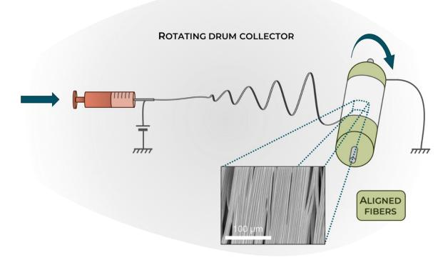
**Figure 1.37 – Effect of a rotating drum collector on the alignment of electrospun fibers** Adapted from Pham *et al.*, 2006 & Chew *et al.*
