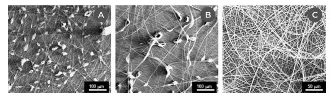
Figure 1.30 – SEM micrographs of electrospun polystyrene fibers obtained from 20 wt/vol% PS solution in (A) THF, (B) CHCl₃ & (C) DMF.
