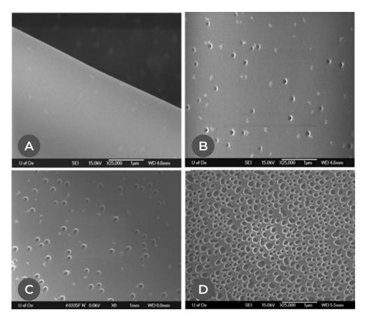
Figure 1.35 – SEM-FEG micrographs of electrospun polystyrene in THF when varying the relative humidity of (A) < 25 %, (B) 31-38 %, (C) 40-45 % and (D) 50-59 %. Adapted from Casper *et al.*, 2004
