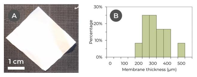
Figure 2.6 – (A) Self-standing PAN membrane after electrospinning (from a 10 wt% PAN in DMF solution) & (B) membrane thickness distribution; N = 12.
