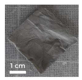
Figure 3.14 – Dual electrospun conductive membrane.
