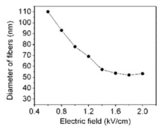
**Figure 1.32 – Dependence of nanofibers diameter on electric field for a PVP/EtOH solution** Adapted from Li & Xia, 2003
