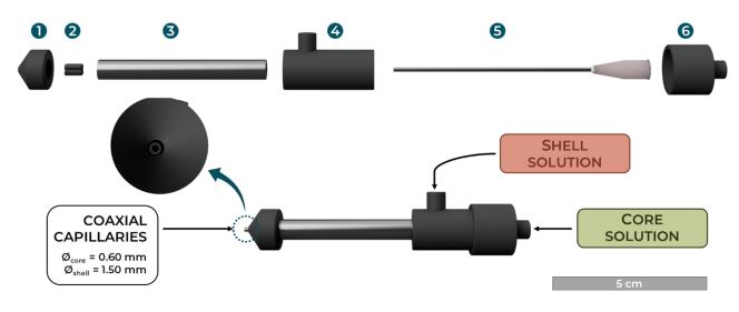
Figure A.2 – 3D-printed coaxial electrospinning spinneret.
