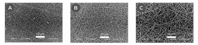
Figure 1.29 – SEM micrographs of electrospun materials obtained from solutions of 34 wt wt/vol% polyamide in 85 vol% formic acid at M<sub>w</sub> of (A) 17 kDa, (B) 20 kDa and (C) 32 kDa. Adapted from Mit-uppatham *et al.*, 2004
