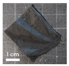
Figure 3.7 – Electrospun PAN 10 wt% + CB 6 wt% membrane.
