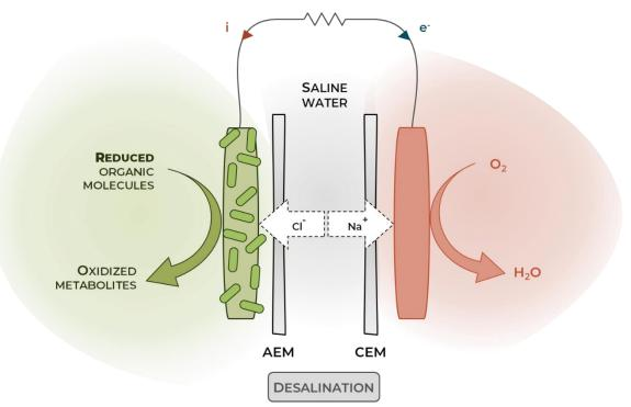
**Figure 1.5 – General architecture of an integrated microbial desalination cell** Adapted from Jacobson *et al.*, 2011
