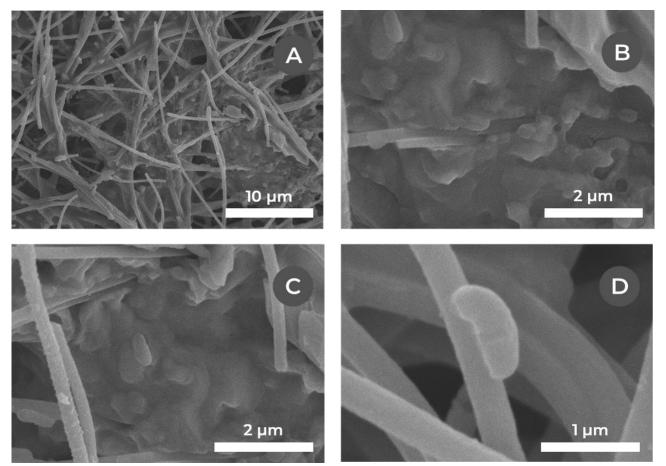
Figure 2.34 – SEM micrographs of an air-dried post-mortem bioanode based on the ex situ precolonized electrospun carbon electrode by *S.* oneidensis after 10 days of operation, polarized at +0.3 V vs. Ag/AgCl, KCl saturated reference, coated with 15 nm of gold. The development of a uniform biofilm between the microfibers is visible.
