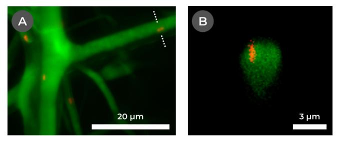
Figure 4.12 – Confocal microscopy of the coelectrospun membrane (shell: PCL 9 wt% + PEG 1 wt% in 90:10 (w/w) chloroform & DMF; core: PEO 5 wt% in PBS 0.5X + mCherry-expressing *P. fluorescens* at  $OD_{600} \approx$  1). Green highlights the Coumarin 6 signal, red the mCherry signal expressed by the bacteria. (A) Micrograph of the coelectrospun fibers colocalized with *P. fluorescens*; (B) Radial cut of one of the fibers and a bacterium along the white dots line.
