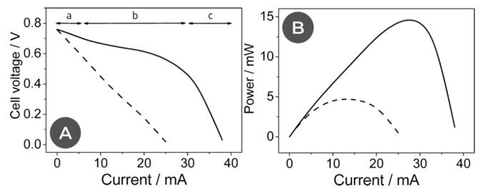
Figure 1.18 – Polarization (A) and power (B) curves of an MFC operating on starch. The solid curves are the original data; the dashed curves represent a mathematically manipulated dataset in which the effect of an increase of the ohmic resistance with 20  $\Omega$  is illustrated. The increase of the ohmic resistance resulted in a linear polarization curve (dashed line). From the slope of this curve and Ohm's law an internal resistance of 30  $\Omega$  can be determined.
