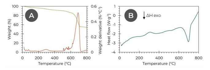
Figure 5.2 – Thermal investigation of the dry residue at 80°C of the wastewater provided by the SIAAP. (A) Thermogravimetric analysis (TGA) of the dry residue. Weight conservation (–) & its derivative (–) against the temperature. (B) Differential scanning calorimetry (DSC) against the temperature. Temperature ramp of 5°C·min<sup>-1</sup>.
