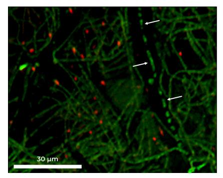
Figure 4.22 – Confocal microscopy of the integrated membrane dyed with Invitrogen<sup>™</sup> LIVE/DEAD<sup>™</sup> BacLight<sup>™</sup> Bacterial Viability Kit (SYTO 9/Propidium iodide). Green highlights live cells while red highlights dead cells. The white arrows show the alignment of live cells along the axis of a coelectrospun fiber (black background; diameter of approximately 9 µm).
