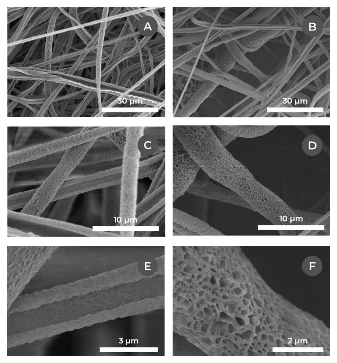
Figure 4.7 – SEM micrographs of coelectrospun fibers (shell: PCL 9 wt% + PEG 1 wt% in 90:10 (w/w) chloroform & DMF; core: PEO 5 wt% in  $H_2O$ ). (A), (C) & (E) Ribbon-like structure; (B), (D) & (F) Round-section fibers. Membrane coated with 15 nm of gold.
