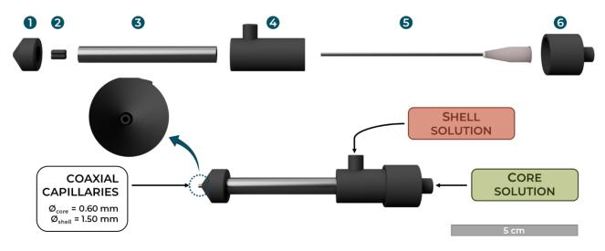
Figure 4.2 – 3D-printed coaxial electrospinning spinneret.
