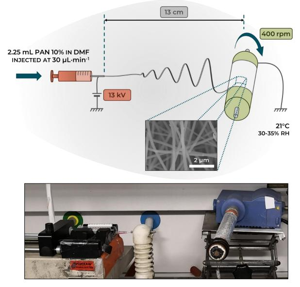
Figure 2.5 - Overview of a PAN electrospinning setup
