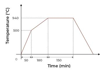
Figure A.4 – Oven settings for the carbonization step.
