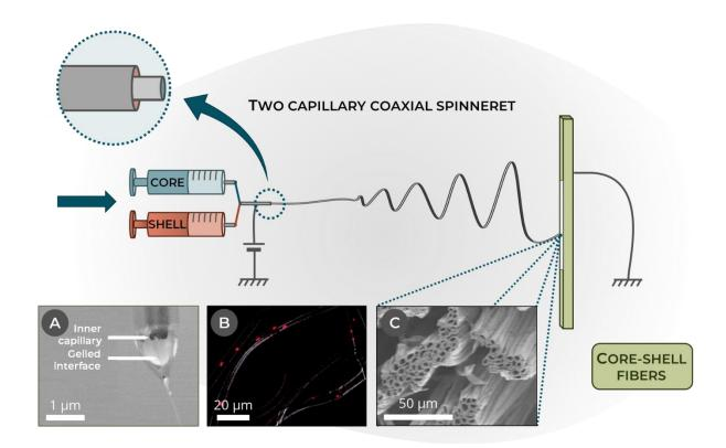
Figure 1.38 – Production of core-shell nanofibers by a coaxial two-capillary spinneret. (A) Compound pendant drop containing a PCL shell and PEO core solution. The protrusion of the inner capillary outside the shell capillary and the gelled interface between the solutions are seen. (B) Fluorescent microscopy of DsRed-expressing *Pseudomonas putida* S12 encapsulated in PCL-shell–PEO-core fibers & (C) High Resolution SEM micrographs of hollow PCL-shell–PEO-core fibers.
