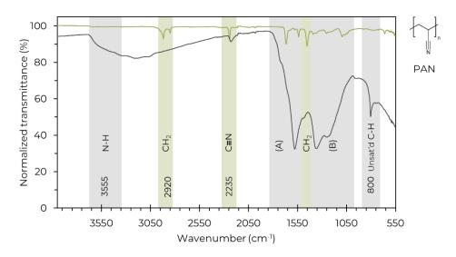
Figure 2.9 – FTIR spectra of raw electrospun PAN membrane (–, from a 10 wt% PAN in DMF solution) and a stabilized membrane (–, under air at 280°C for 3 hours). The two heavy bands in the stabilized membrane spectrum correspond to (A) conjugated double bonds, C-O, N-H & O-H & (B) C-O-C bending and C-O stretching, both characteristic of the oxidized and cyclized stabilization products. A blank was recorded and subtracted from the presented spectra.
