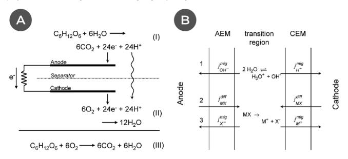
Figure 1.21 – Effect of ion exchange membranes in MFCs with (A) a simplified model of the redox reactions and charge-balancing ion transfer in an MFC and (B) a schematic illustration of the structure of and the ion fluxes across a bipolar membrane.
