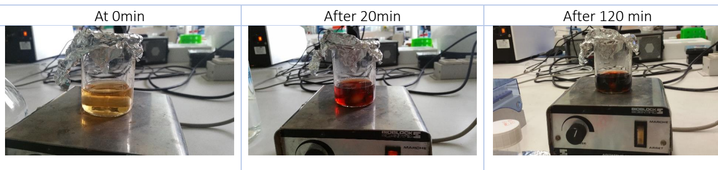
Figure 3: Color change of the dopamine solution in presence of sodium periodate as a function of time
