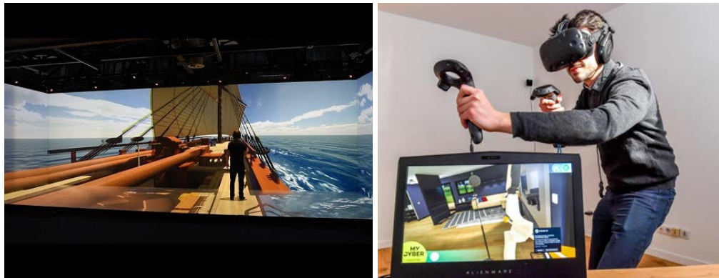
Figure 1.1 – Examples of the two main visual display systems to experience VR. Left: A user immersed in the Cave Immersia in Rennes, France. Right: A man uses an HMD and joysticks at the MCR offices in Lille, France. Philippe Huguen / AFP - Getty Images file
