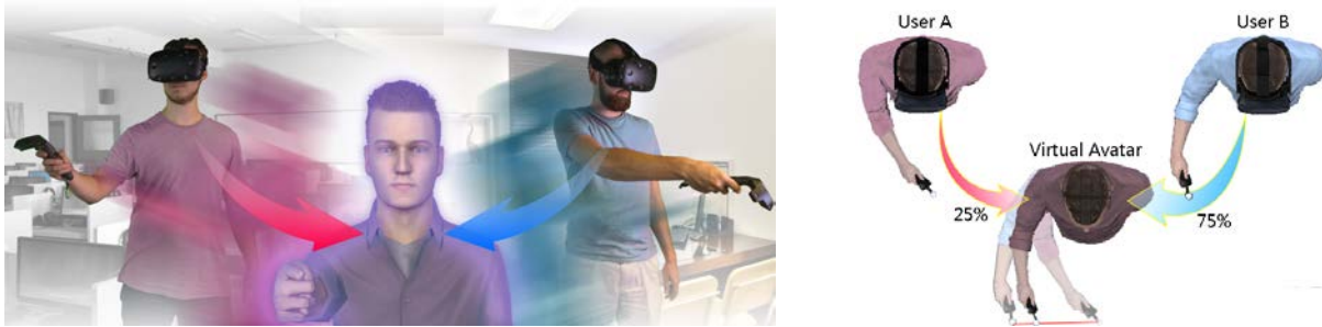
Figure 4.1 – Our “Virtual Co-Embodiment” experience enables a pair of users to be embodied simultaneously in the same virtual avatar (Left). The positions and orientations of the two users are applied to the virtual body of the avatar based on a weighted average, e.g., “User A” with 25% control and “User B” with 75% control over the virtual body (Right).
