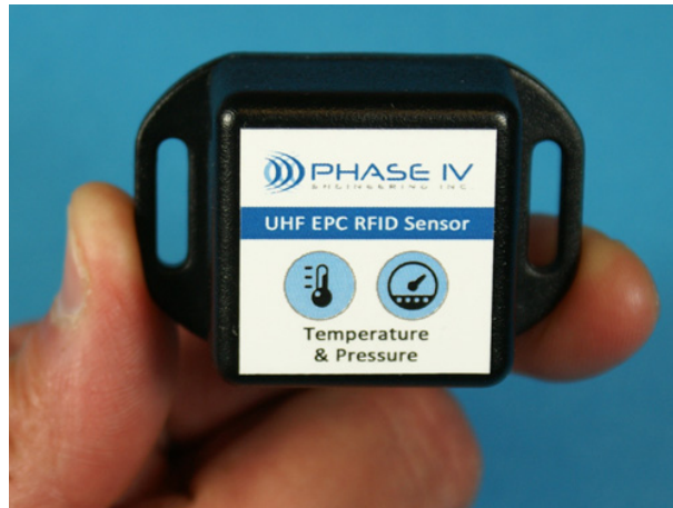
FIGURE 1.8 – Exemple de tag UHF de PHASE IV Engineering [2]
