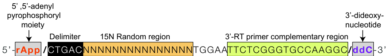
Fig. 2 Sequence details for the 3'-Adap adapter. 3'-Adap is a preadenylated oligonucleotide containing a 5',5'-adenyl pyrophosphoryl moiety (see Note 4 ). The delimiter sequence allows for the demarcation between the sequence corresponding to the 3' end of the RNA and the adapter sequence. This sequence is also used during bioinformatics analysis to discriminate read 2 containing adapter sequence from other sequences that could arise from artifacts of reverse transcription priming (Fig. 4). The 15 random bases (15 N) allow for deduplicating and therefore for eliminating PCR duplicates. The 3'-RT primer complementary region is used as template during reverse-transcription reaction. Finally, the 3'-dideoxynucleotide prevents the 5' adenylated oligo from self-ligation
